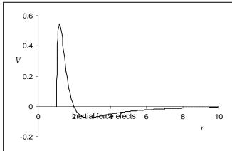
Fig. 4b. Azimuthal velocity at B = 0.66,  $\theta = \pi/2$ . For 1/3 < B < 1, elastic forces dominate near the sphere surface and inertial forces dominate away from the sphere
