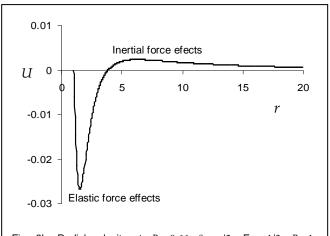
Fig. 3b. Radial velocity at B = 0.66,  $\theta = \pi/2$ . For 1/3 < B < 1, elastic forces dominate near the sphere surface and inertial forces dominate away from the sphere.
