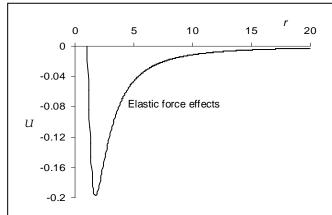
Fig. 3c. Radial velocity at B = 2,  $\theta = \pi/2$ . For  $B \ge 1$ , elastic forces determine the nature of the radial velocity profiles.
