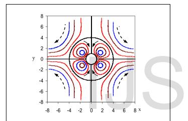
Fig. 2b. Stream lines at B = 0.66. Elastic forces dominate near the sphere surface and inertial forces dominate away from the sphere
