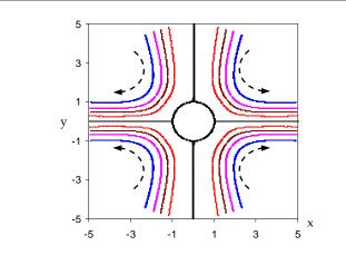
Fig. 2a. Stream lines at B = 0.3. Inertial force caused fluid to be thrown outward centrifugally at the equatorial zone.
