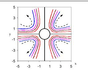
Fig. 2d. Stream lines at B = 3. For B > 2, the shape of the streamline become independent on B.
